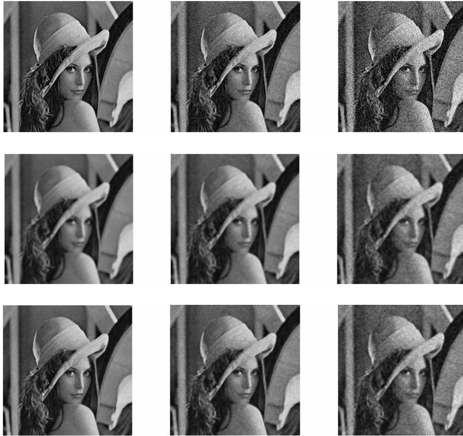
Fig. 16. First row shows the input images. Second row is the output of bilateral filter with window size of 5, \sigma_d=2 , and \sigma_r=10 . Third row is the output of the new filter with window size of 5 core size of 1, \sigma_d=2 , and \sigma_r=10 . The additive noise is Gaussian and in the first column its \sigma is 8, in second column 16 and in third column 32.
