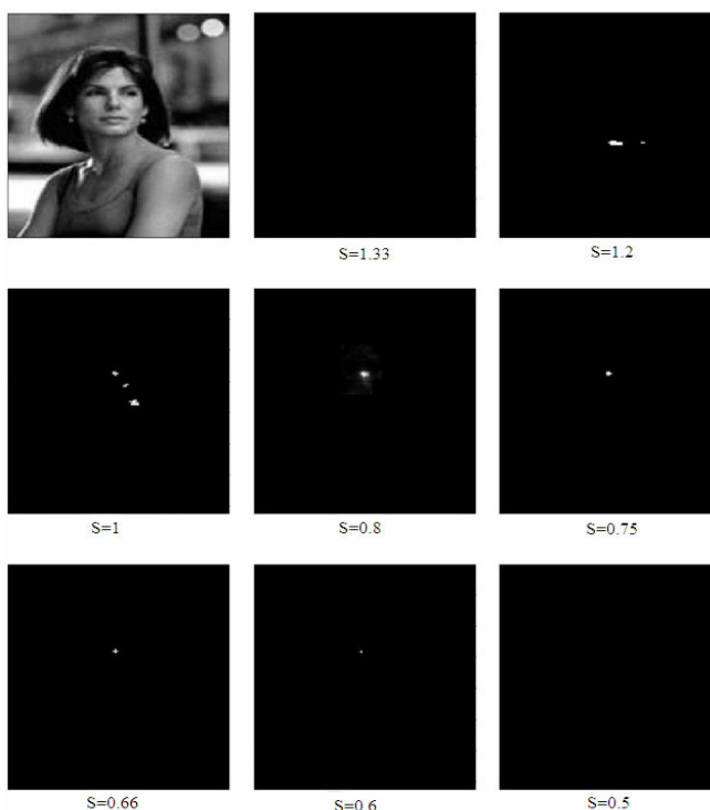
Figure 8: Final face detection based on detection results of sequent scales. A face pattern is detected in scale=0.8 and scale=0.75.
